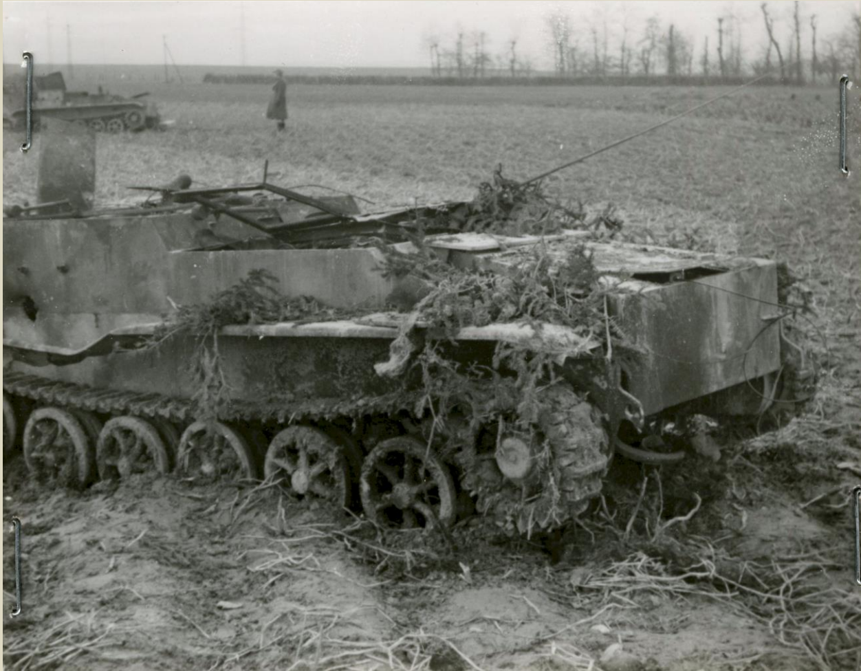
Photo 2. Right side. Note hit one side of engine compartment.
