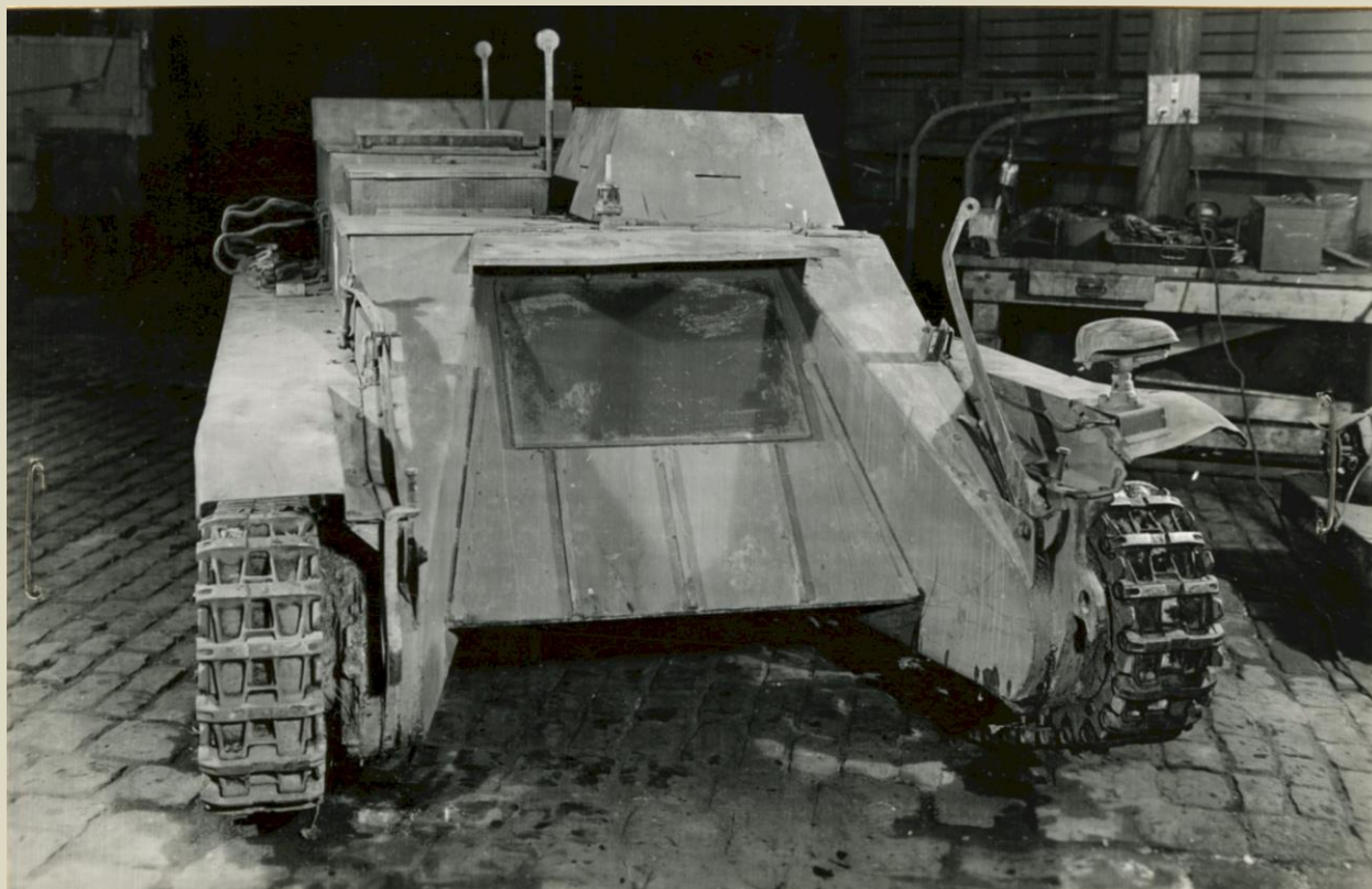
Photo 2: Front view showing the hatch over the differential and arms of the charge release mechanism.
